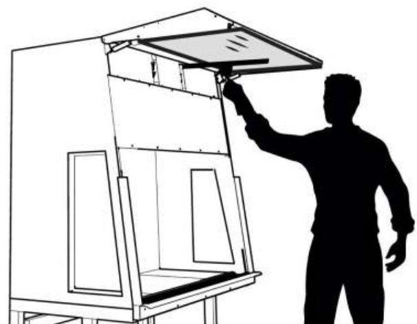
Cleaning the front window
