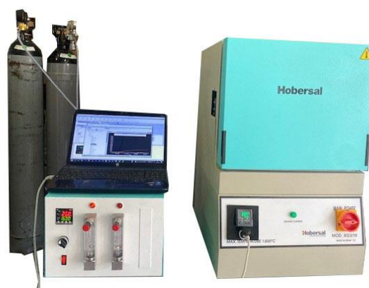
XG3+ automatic Gas supply system controlled by Eurotherm EPC3016 + Itools software
